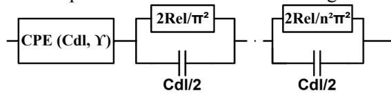
Figure 8. CPE model equivalent circuit [4]
