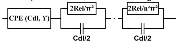
Figure 8. CPE model equivalent circuit [4]
