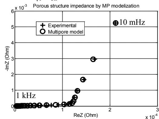
Figure 7 Porous structure impedance MP model fitting
