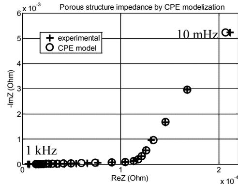
Figure 6 Porous structure impedance CPE model fitting
