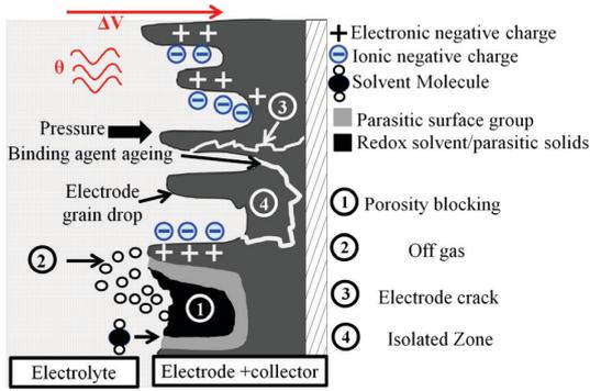
Figure 1. Ageing causes and effects of EDLC
