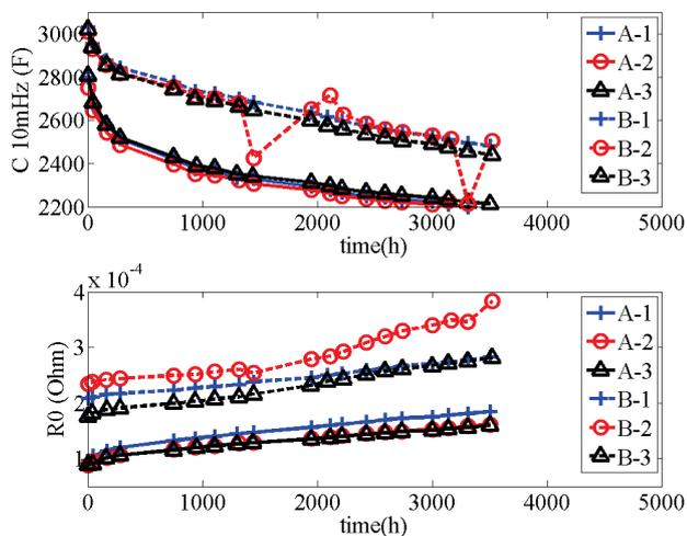
Figure 8 EDLC parameters evolution with ageing
