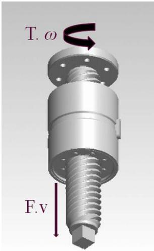
Figure 2.4. Roller screw with torque and force.
