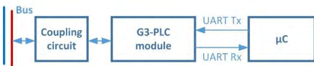
Fig. 10 Communication schema based on G3-PLC protocol
