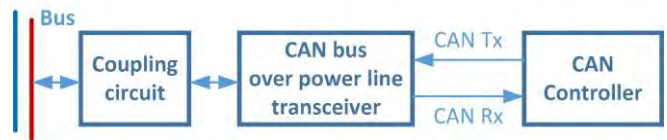
Fig. 11 Communication schema based on CAN protocol
