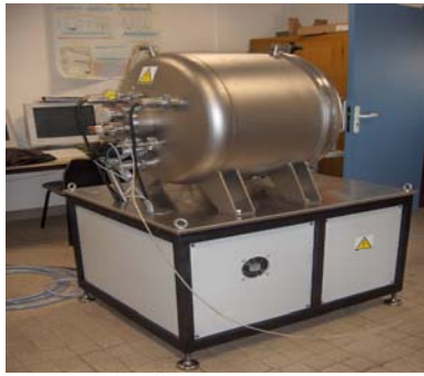
Fig. 3: Picture of the high temperature chamber enabling high temperature electrical measurements (25 °C → 600 °C).
